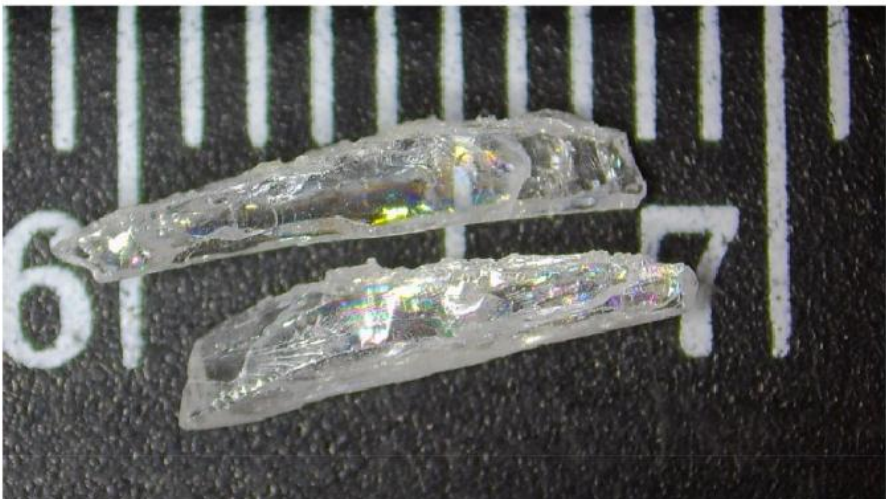
FIG. 12. (\text{Pb}_{0.5}\text{Sr}_{0.5})\text{WO}_4 single crystal produced by the crystallization in the solution of \text{PbWO}_4 .
